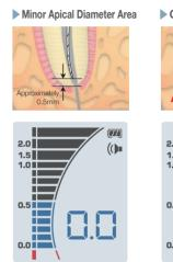
When the tip of the file reaches the minor apical diameter, the bar graph display reads 0.0, and the alert sound changes to a continuous tone
